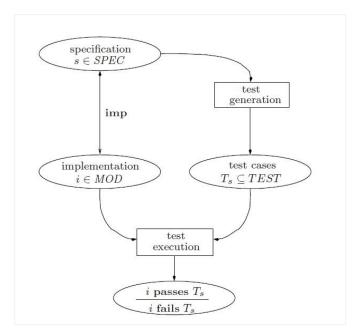
Figure 5. The formal, specification based testing process
