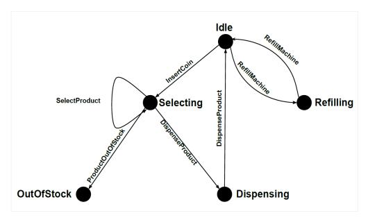
Figure 4. LTS illustration of a simple vending machine
